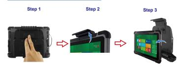
1.Slide the latch to open the hook
