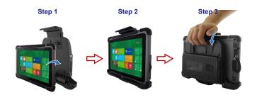
1 Insert the Tablet PC into the docking
